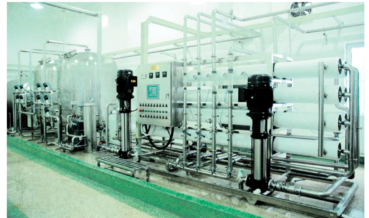
香港康琪壹佰有限公司 15m 3 /h二级反渗透纯化水系统 15m 3 /h two-stage reverse osmosis purified water system of Hongkong Kang Q.Y.Bai Biological Technology Co., Ltd.
