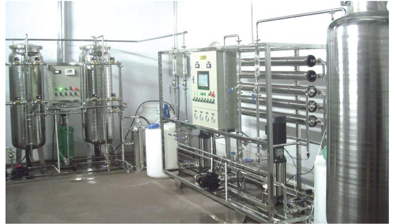
辽宁大石药业有限公司 (辽宁本溪北方药谷) 1m 3 /h二级反渗透纯化水系统 1m 3 /h two-stage reverse osmosis purified water system of Liaoning Dashi Pharmaceutical Co.,Ltd. (Beifang Medicin Valley,Benxi ,Liaoning)
